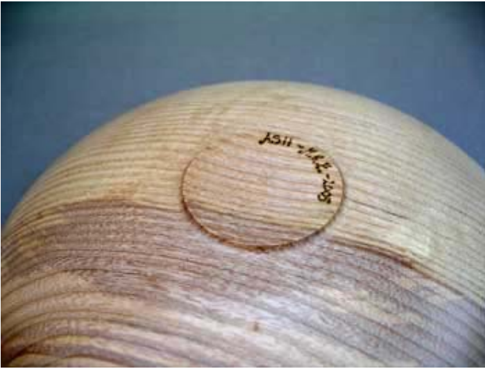
21. The finished foot. Apply the liming paste to the outside of the bowl and protect with your choice of finish. I used Liberons finishing oil.
