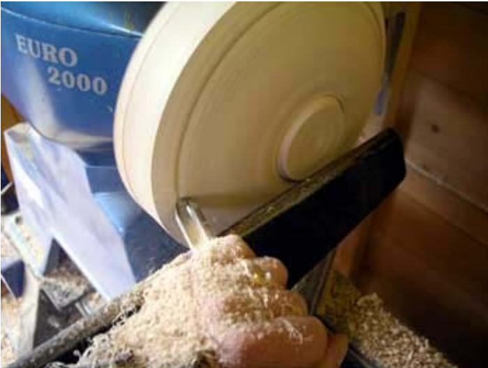
3. Here the back of the bowl is starting to be shaped. A 60mm spigot has been cut using a parting tool in preparation for the O'Donnell jaws.
