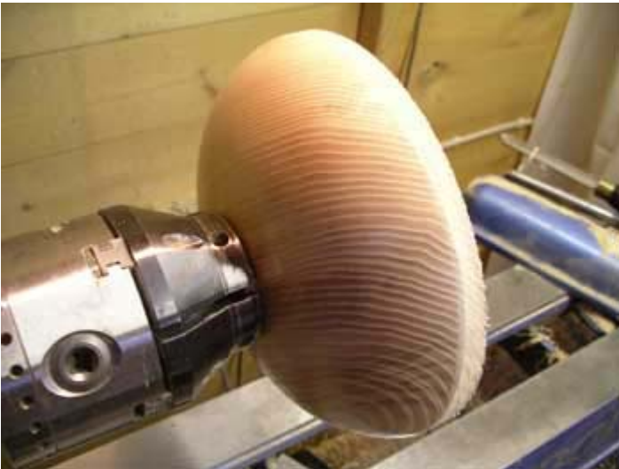
7. Here the faceplate has been removed and the bowl is now being held in the Axminster Super Precision chuck using the O'Donnell jaws. These jaws give greater clearance when working near the jaws.
