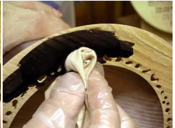
16. Applying the stain with a piece of cloth. I use a water based pre-mixed wood dye. Try not to spill it!
