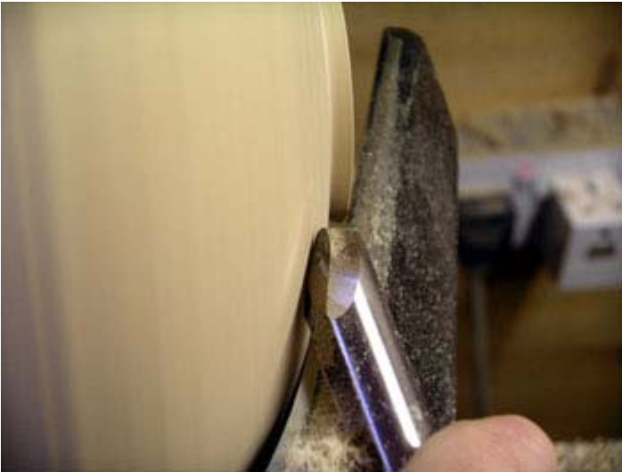
5. A shear cut is made on back of the bowl using the 1/2" bowl gouge. Notice the cotton wool type shavings below the tool. This cut will remove any tearing of the grain caused by the roughing cuts.
