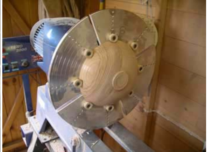
20. The large Axminster button jaws are used to reverse chuck the bowl so that the bottom foot can be finished.
