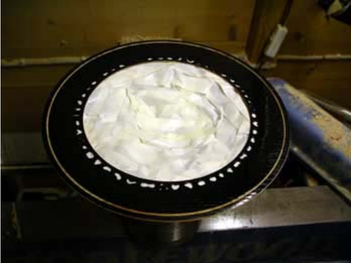
19. The inside is masked off and aerosol based sanding sealer and then satin acrylic lacquer is applied.
