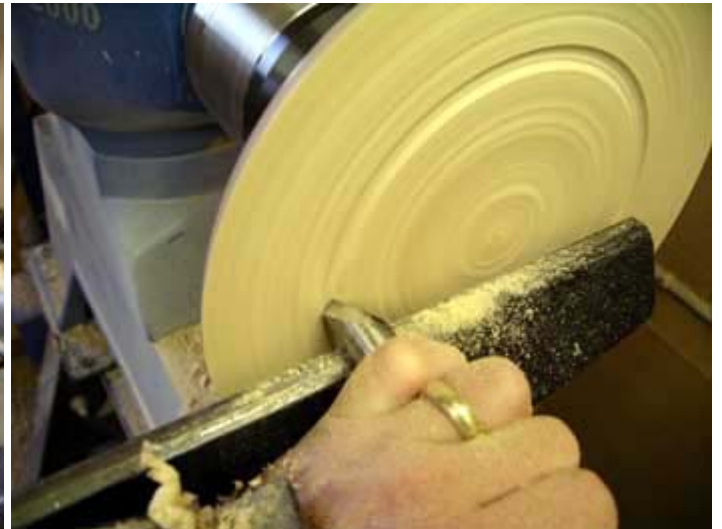
8. Again using the 1/2" bowl gouge the top side is levelled and the correct depth attained.
