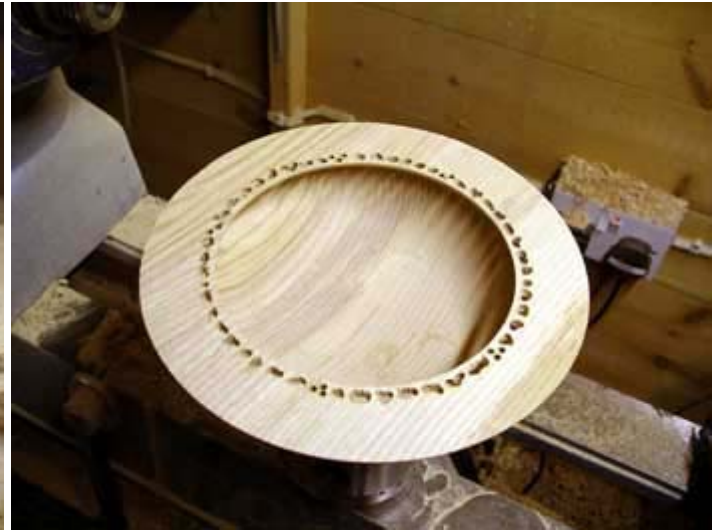
14. The piercing is now completed. Note: I removed the whole chuck from the lathe rather than removing the bowl from the jaws. This is so that the bowl does not move which can happen when re-chucking.
