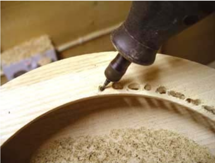
13. Cut the holes using a Dremel (or similar) tool with an 1/8" burr attachment. I used a completely random pattern but you can do whatever you want.
