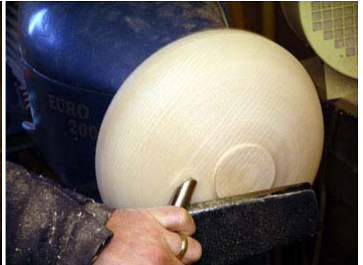
4. The shape of back of the bowl is being finalised with the 1/2" bowl gouge.
