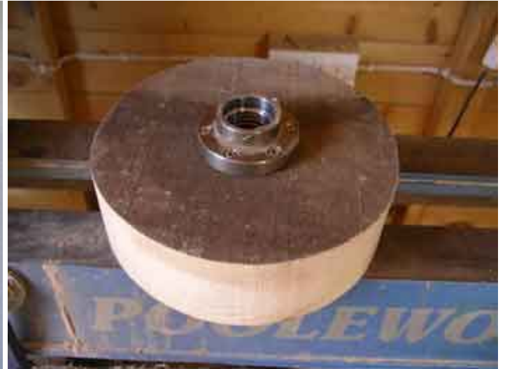
2. The timber of choice is English Ash 9" x 3". Here the piece is shown with the 3" face plate ready to be screwed on to my Poolewood Euro 2000 lathe.
