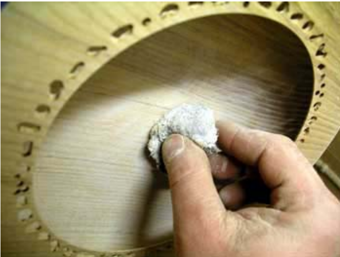
15. Here I am using Liming Paste to enhance the contrast with the black rim and accentuate the grain.
